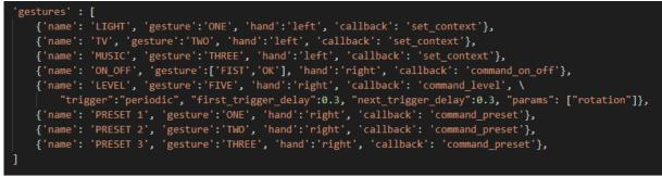
Note the parameter 'trigger' for the gesture named 'LEVEL'. The value 'periodic' means that an event will be sent every 0.3s (value of 'next\_trigger\_delay') as long as the user is doing the FIVE gesture. When 'trigger' is not specified, as it is for other gestures, the default behavior is to send only one event to the client.
