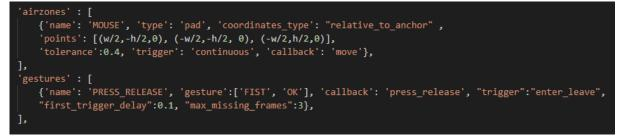
'coordinates\_type': "relative\_to\_anchor" in the airzone definition, means that the following 'points': [(w/2,-h/2,0), (-w/2,-h/2, 0), (-w/2,h/2,0)] are coordinates relative to an anchor point, instead of the camera origin.
