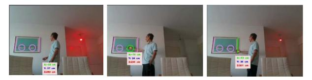
c. The **pad** is a « flat » parallelepiped defined by a foundation plane given by 3 of its points (P<sub>1</sub>, P<sub>2</sub> and P<sub>3</sub> on the schema below) and a perpendicular depth 'tolerance'. A hand inside the parallelepiped can be projected onto the foundation plane. The projection has a position (x, y) in the coordinate system (origin P<sub>1</sub>, P<sub>1</sub>P<sub>2</sub>, P<sub>1</sub>P<sub>4</sub>) :
